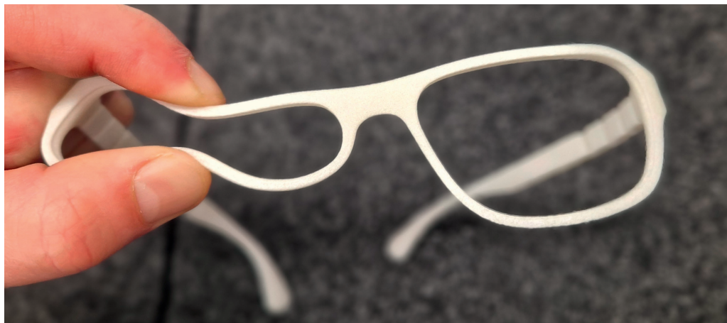
Improved mechanical properties of PA12 parts as a result of closing the laser-sintering material loop. © Oerlikon AM Europe GmbH
